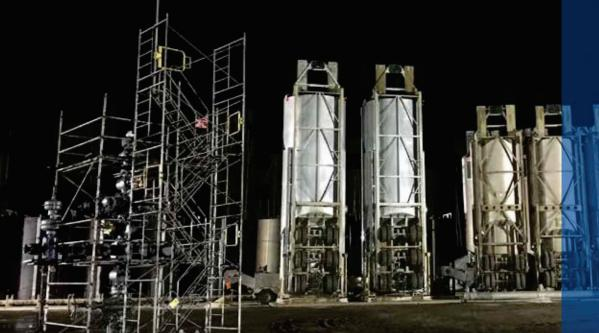
Our reputation for innovation started with our silo systems: The Propmasters. This one-ofa-kind self-standing silo storage system relies on our patented technology to drastically reduce the on-site space necessary for sand storage.
